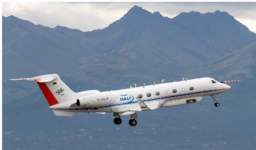
Measurement flight start of HALO. Various air inlets are visible at the top, and the belly pod with the remote sensor GLORIA can be seen below the fuselage. (Copyright: Andreas Minikin/DLR)
