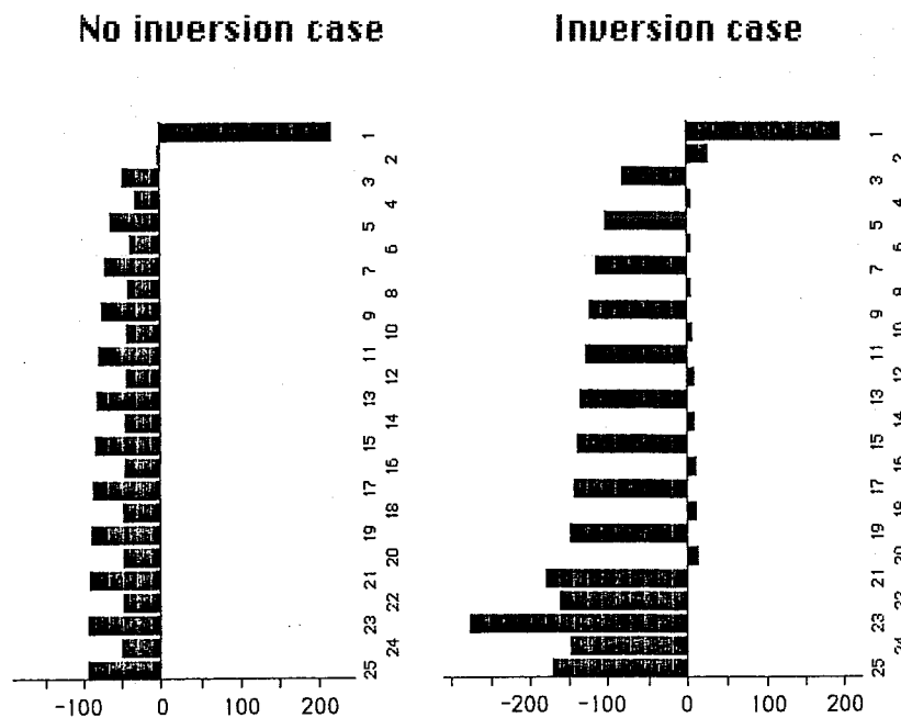
Fig. 3. Errors of the Nested Grid Model (see text for details) pressure gradient force scheme, for the "no inversion case" (left hand panel), and the "inversion case" (right hand panel), for a vertical structure of 25 sigma layers of equal thickness. Values are given in increments of geopotential ( m^2 s^{-2} ), between two neighboring grid points, along the direction of the increasing terrain elevations.
