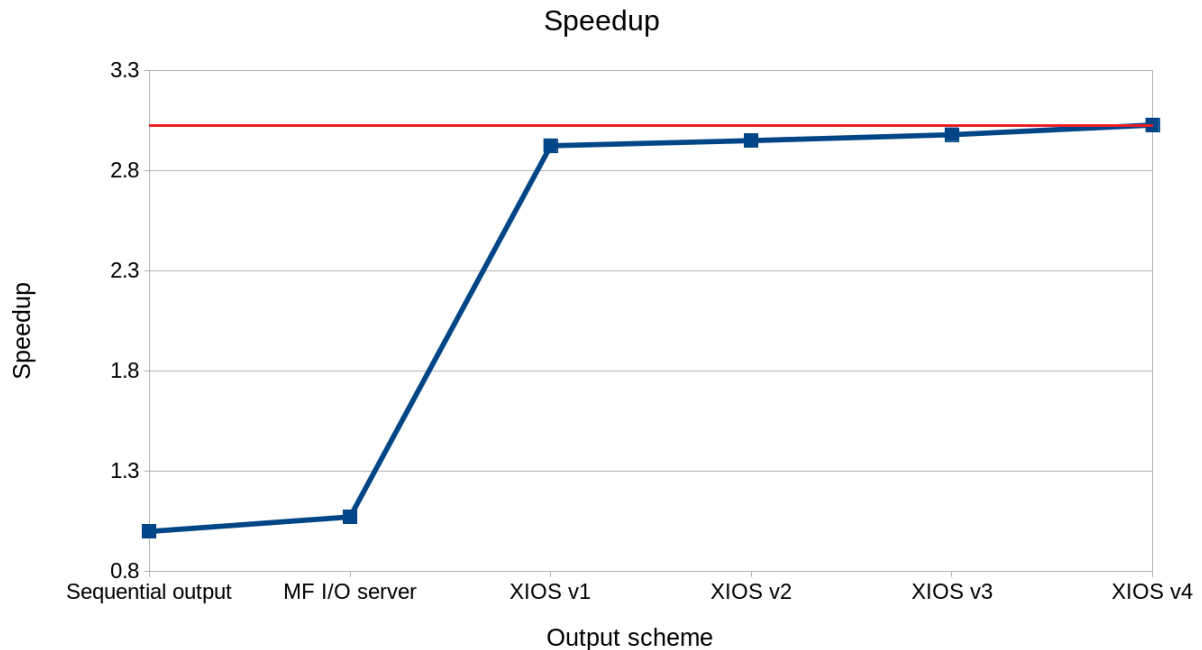
Figure 30: Comparison of the speedup of different output schemes, where both sequential output and MF I/O server have the additional cost of converting GRIB to netCDF files
